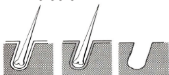
Fig. 2. Action of unhairing agent during a hair-saving system
